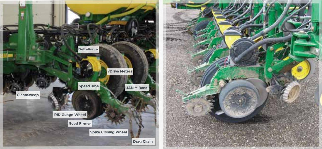
Figure 8: Planters equipped for planting into cover crops.
