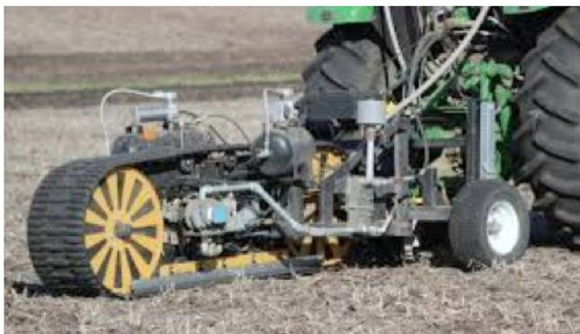
Figure 1. Autoprobe soil sampling machine (<http://www.agrobotics.com>).
