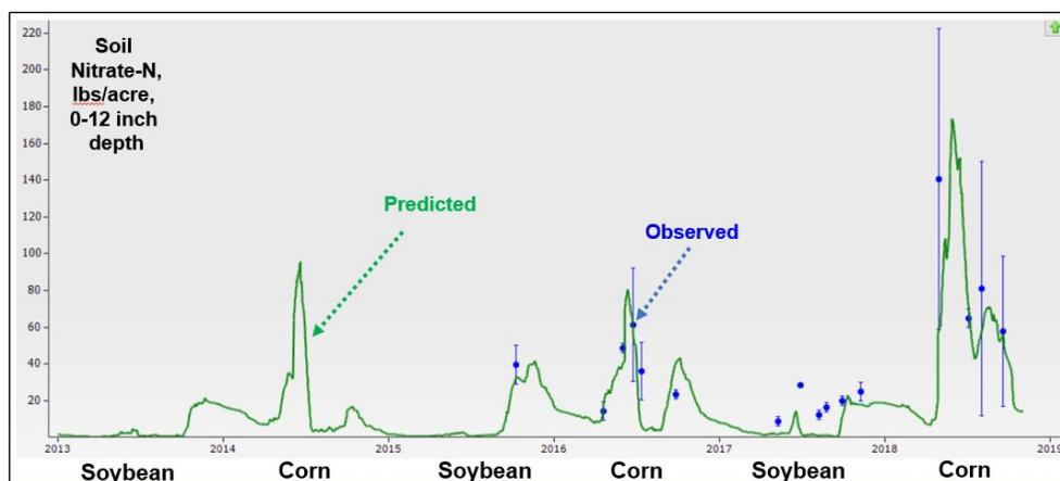
**Figure 1. Calibration of APSIM model using the observed soil nitrate-N data sampled during 2016, 2017 and 2018 growing seasons with cover crop. The vertical bars are variation for each sampling date. The spikes in the predicted soil nitrate values result from manure, commercial N fertilizer applications and mineralization of soil organic matter over several growing seasons.**
