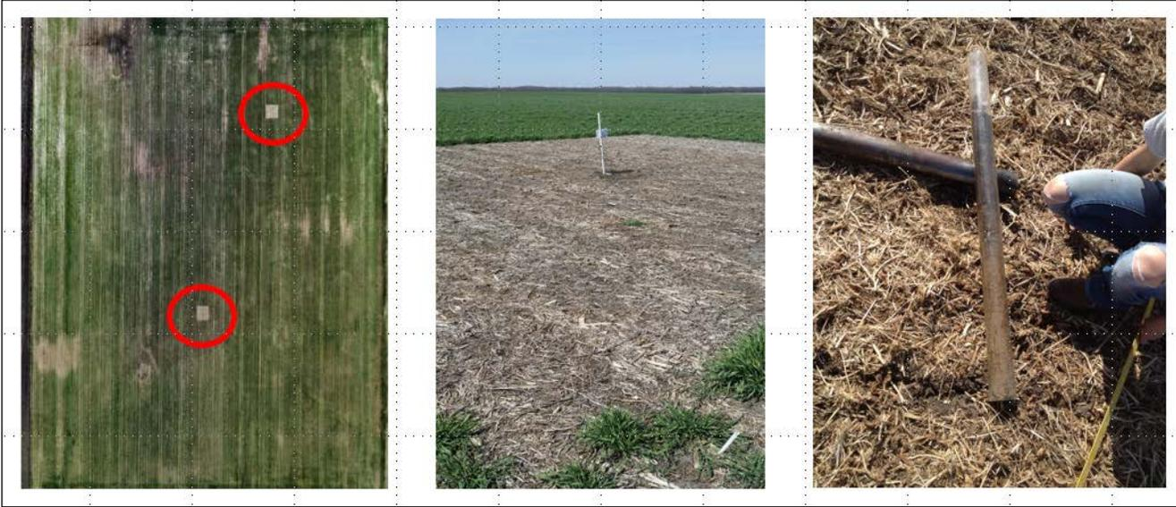
Figure 3. Left: Two control areas without cover crops in a farmer’s field with tile drainage. Center: Soil and moisture sensors at the control area. Right: Soil cores taken at 0–36 inches to develop a digital soil profile for modeling simulations.
