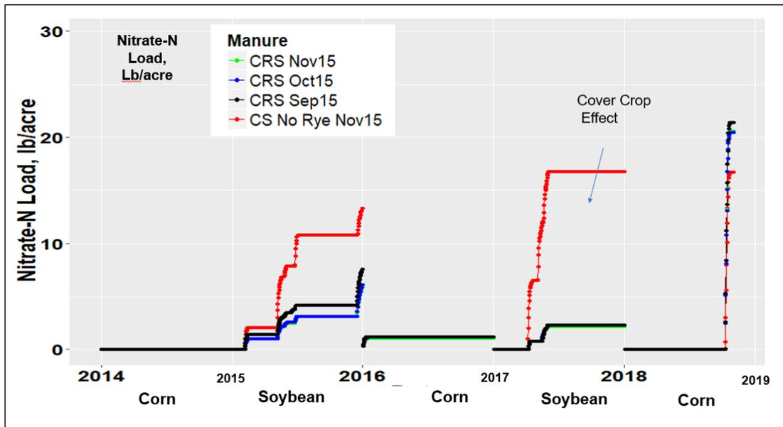
Figure 4. Nitrate loss from four simulation scenarios with different timing of fall swine manure applications with or without cover crop.
