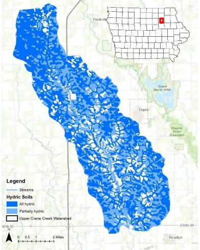
Figure 2.5.2. Soil map units in the Upper Crane Creek Watershed that are classified as hydric.
