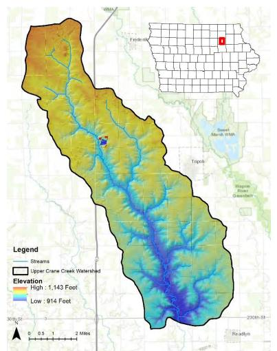
Figure 2.4.1. LiDAR-derived elevations within the Upper Crane Creek Watershed.
