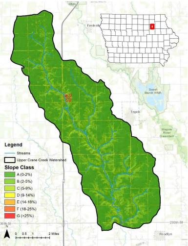
Figure 2.4.2. Upper Crane Creek Watershed slope classifications derived from elevation data.
