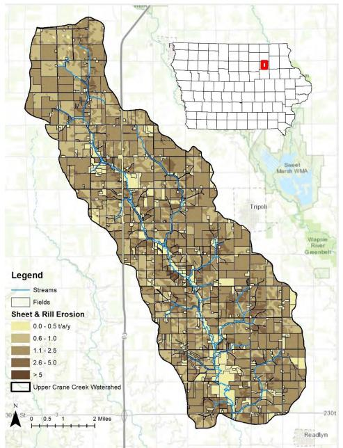
Figure 2.9.1. Estimated sheet and rill erosion rates based on soil types, topography and land use in the Upper Crane Creek Watershed.
