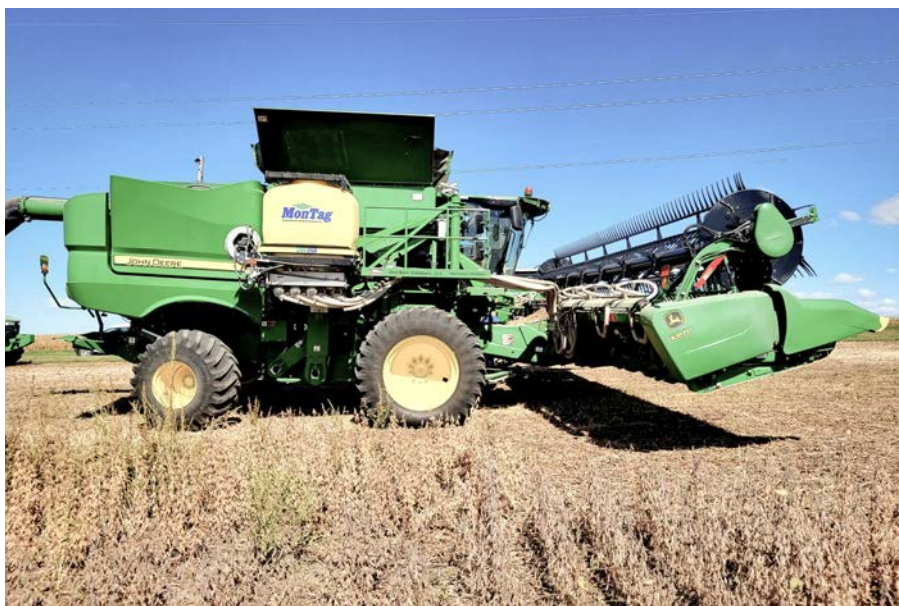
Figure 1. Red Barn Solutions' Harvest Seeder, a combine-attached air seeder.
