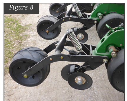
Figure 8. Two small disc closing wheels shatter sidewall compaction in this after market product.
