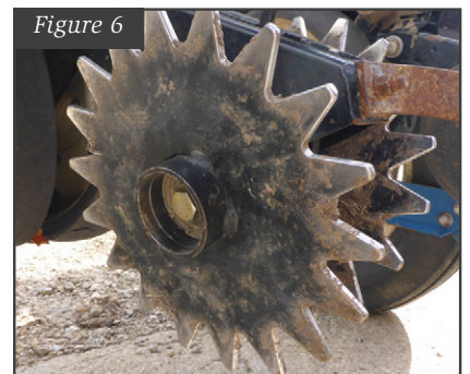
Figure 6. Spike toothed closing wheel.
