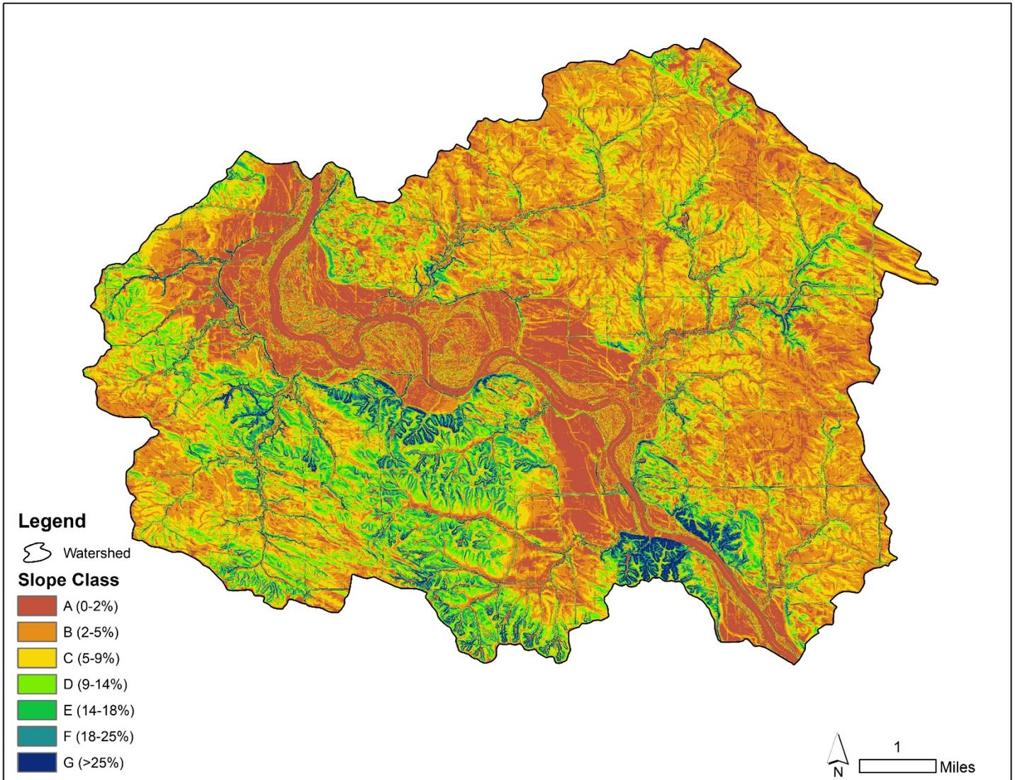
Figure 2.4.2. Slope classifications in the Mill Creek Watershed derived from elevation data.
