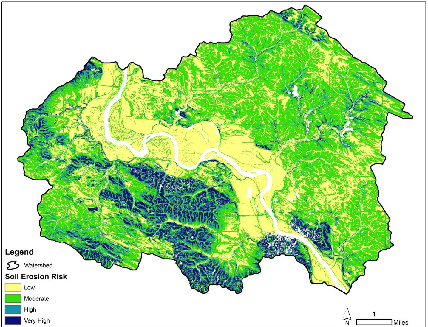
Figure 2.5.4. Soil erosion risk naturally varies throughout the watershed based on topography and soil properties.
