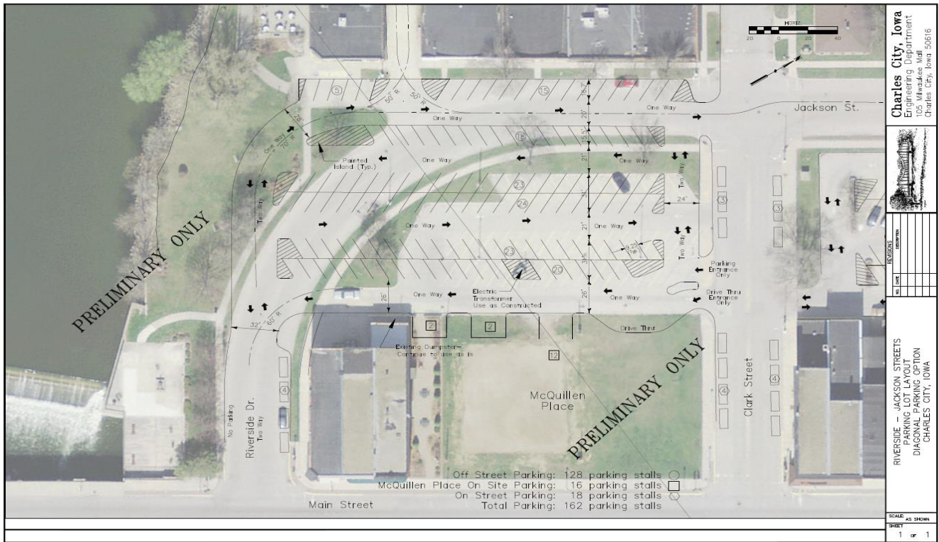
Figure 5.2.3. Potential layout of new parking lot at Jackson Street in Charles City with integrated LID practices.
